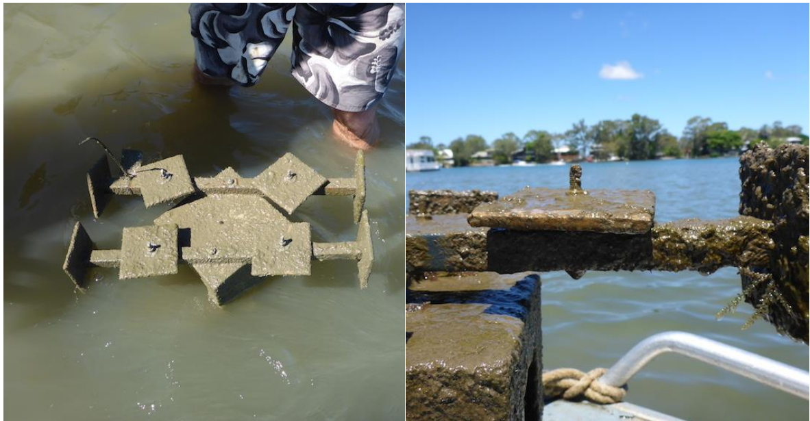
Figure 13. Sediment smothering upper horizontal surface of settlement tiles after 2 months
